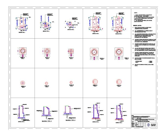
The width/diameter of the manhole should not be less than internal diameter of the Drain + 150mm benching on both sides (150mm + 150mm).
