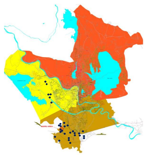
Fig 5.1: Map of Srinagar City showing proposed SWD Missing Links (1) sites/areas (Symbolic Blue Dots- showing SWD sites for reference)
