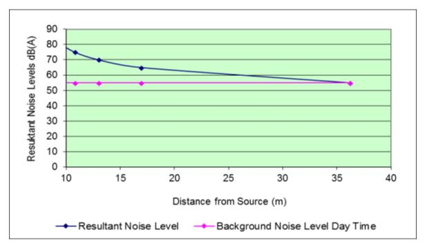
Figure 6.2: Attenuation of Noise Level During Construction Stage
